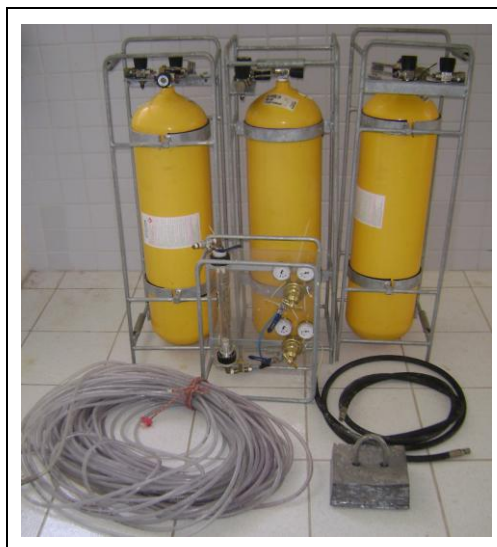
Figure 3 – Set of used equipment for gas release into the sea bottom.
