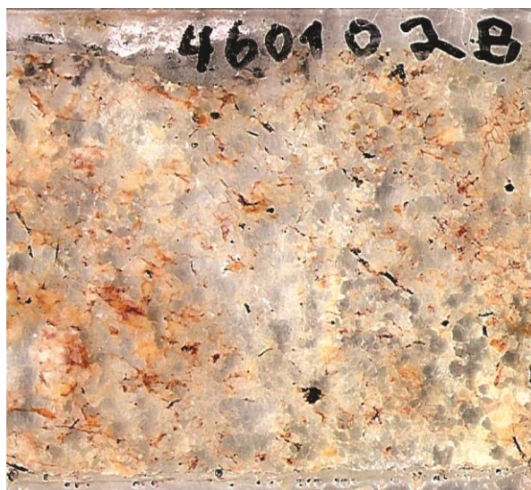
Figure 5 Polished thin section HB 460102B, of the banded sodic aplite from the Picuí pegmatitic-granite bench. Black dots are mostly xenotime and zircon and some magnetite. The fine alternance of pink and beige bands simulating the garnet bearing “line rocks” in this case is given by variation of proportions of feldspar and quartz. The pink colored bands are the result of very fine impregnation of limonite at the borders and fractures of well-rounded quartz grains, macroscopically possible to be suspected to be garnet. Beige bands are richer in feldspars and low hydroxide impregnations.
