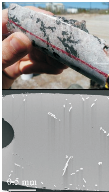
Figure 6- Dendrites of manganotantalite in the Tanco pegmatite (up) and in an experiment at 1000°C (down) supercooled by 250°C in 3 min.
