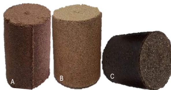
Figure 3. Briquettes made from açai (A), cupuaçu (B), and murumuru (C) with a grain size of 60 mesh (0.245 mm) subjected to a pressing time of 15 minutes. This image showcases the compacted biomass products after the briquetting process..
