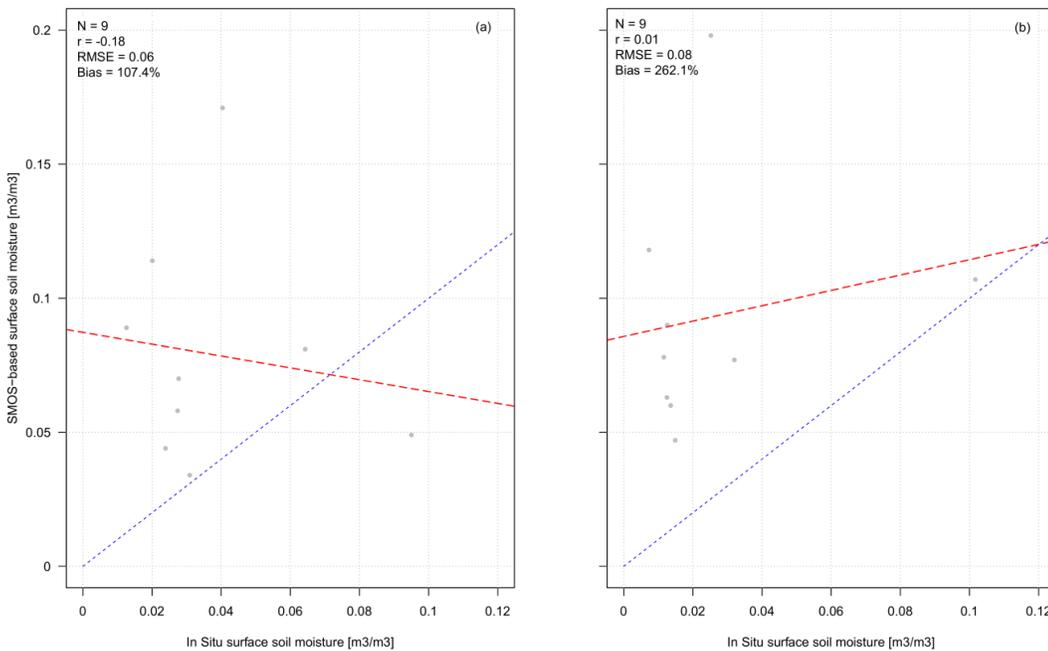
Figure 3 – As Figure 2, but for the SSM retrieved from SMOS, **(a)** the A1 site; and **(b)** the A2 site. Dashed blue line indicates 1:1 correspondence. RMSE is the root mean squared error in the same units of the SMOS SSM and in situ SSM, and Bias is the percentage of bias between both variables.
