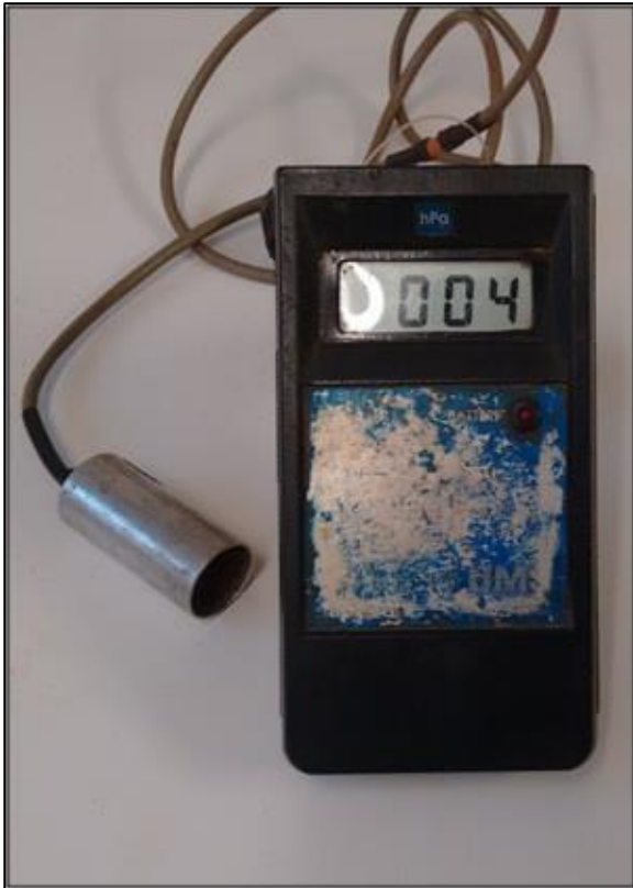
Figure 5: INFIELD 5 tensiometer, used to measure the matric potential. Source: Authors, 2017.
