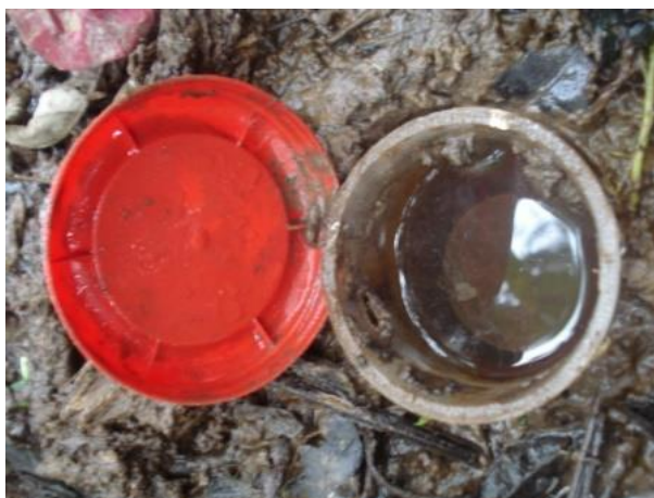
Figure 3. Detector filled with surface runoff water after a rain event.
