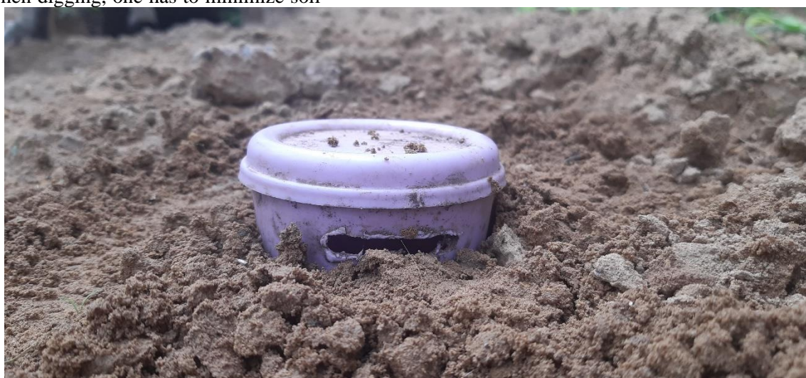
Figure 2. Surface runoff detector installed on the soil surface. Note the hole of the detector is leveled relative to the soil surface.
