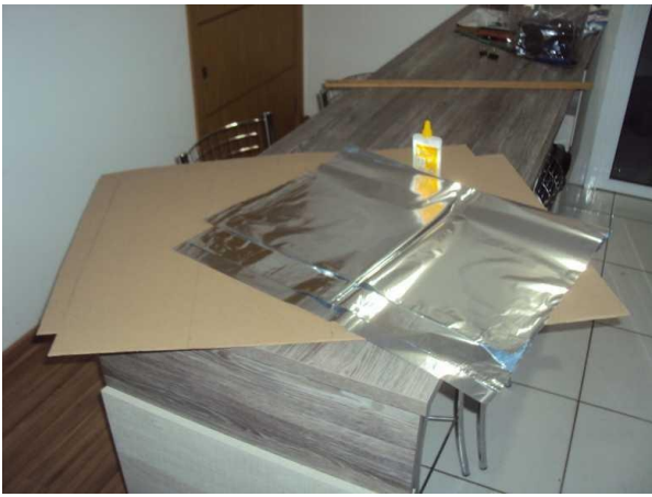
Figure 6. Cardboard sheets and metallized BOPP plastic reflexive sheets. Source: The authors.
