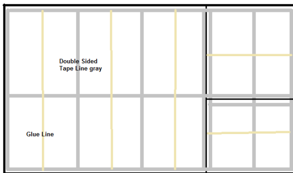
Figure 7. Schematics on double sided tape and glue line to glue reflexive the sheet on the cardboard. Source: The authors.
