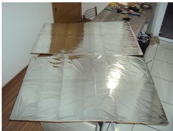
Figure 11. Two cardboard sheets covered with reflexive films. Source: The authors.
