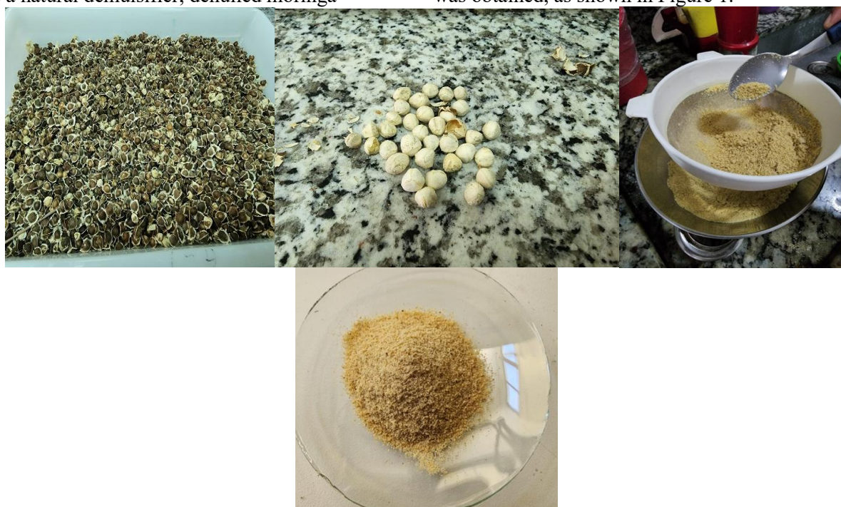
Figure 1. Moringa seed processing process to obtain powdered coagulant.
