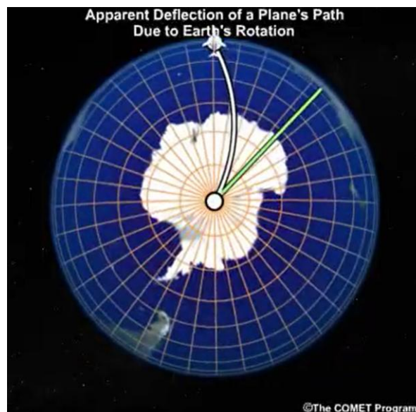
Figure 7 An airplane departing from the South Pole is flying in a straight line, aiming to reach the equatorial latitude indicated by the green line. However, as the Earth rotates beneath the airplane, it appears to be deflected to the left relative to the Earth's surface (white curve). Adapted from The COMET Program (s/d).
