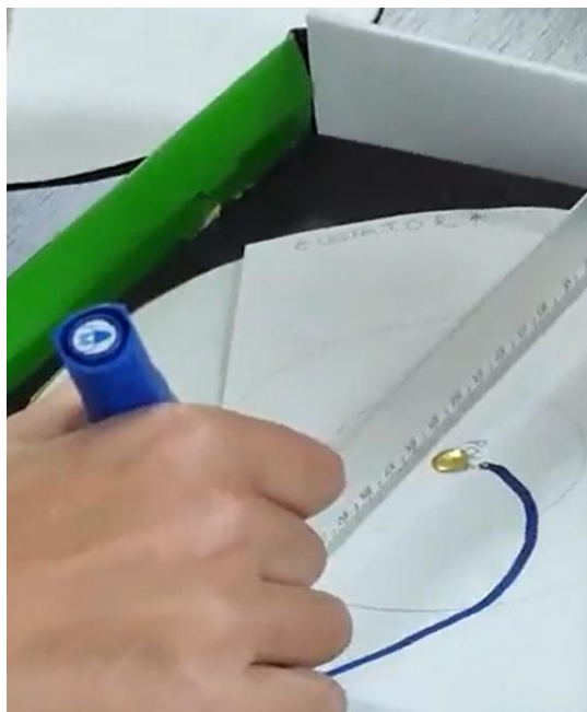
Figure 4 Curved trajectory on the rotating disk. When the disk is rotating, and we attempt to draw a straight line following the ruler, the resulting line appears curved. Details about the direction of rotation are provided in the next sections.
