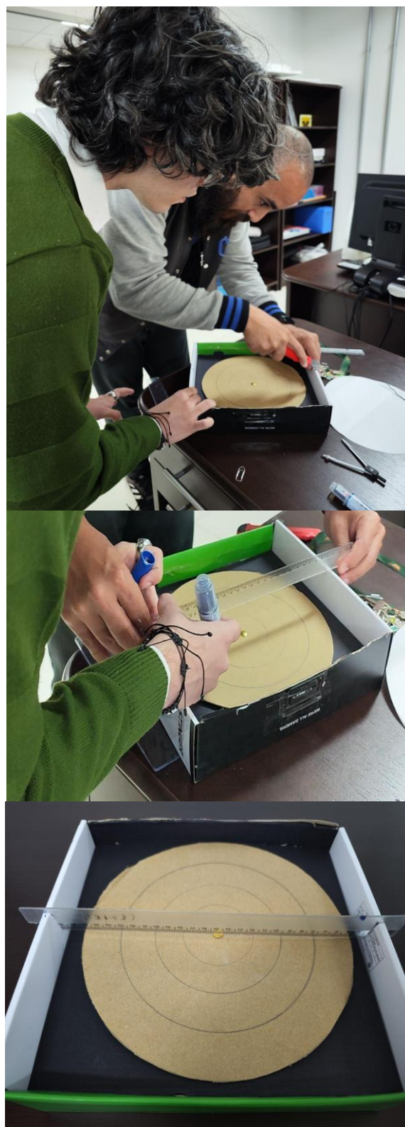
Figure 3 A paper-based model of a rotating surface is being constructed. A cardboard disk is fixed with a pin to the box, and a ruler is also secured to both sides of the box.
