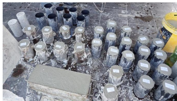
Figure 6 – Concrete production (test specimens).
