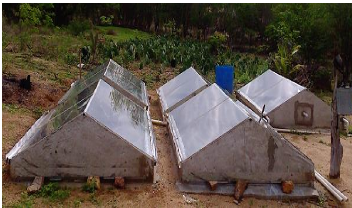
Figure 2 - Solar desalinizers installed in the Olho D'Água settlement, Seridó-PB.
