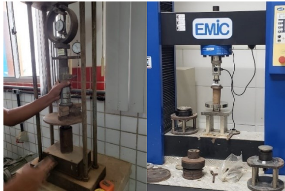
Figure 2 - Simple compression test: static molding (a) and breaking of specimens (b), Recife, Pernambuco.
